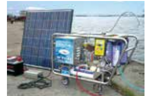
Power supply is secured by solar panels.
